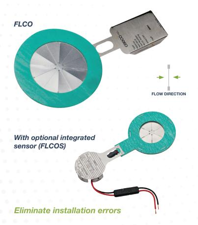
OsecoElfab's FLCO rupture disc is easy to install and non-torque sensitive. The disc fits between standard 150# ANSI RF flanges with no need for a holder. As a flat, bi-directional device with the same burst pressure in either direction, the FLCO cannot be installed incorrectly, eliminating installation errors.
